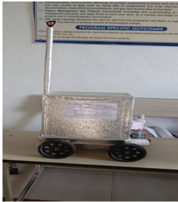
Figure 7.5.3: Self-navigating, monitoring and garden maintenance robot for water sprinkling & lawn cutting
