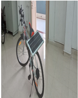
Figure 7.5.4: Solar Electric Bi-Cycle with smart Battery and Theft Detection
